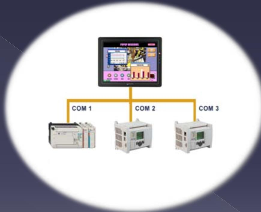
Every MT8000 HMI supports 3 serial ports. With this feature, users can connect multiple devices simultaneously – including PLCs other than the S7-1200, drives, controllers, bar code scanners and more.
